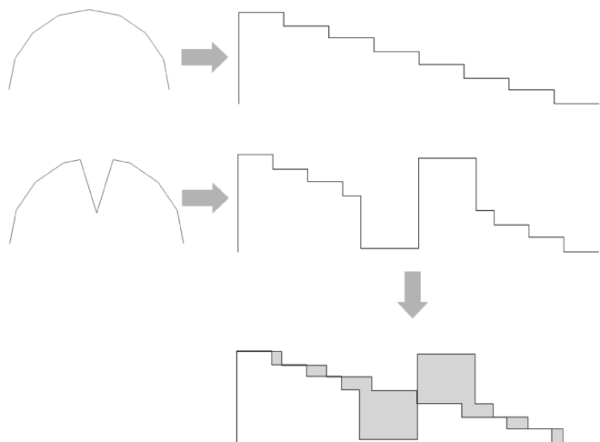
Fig. 3. Two polygonal curves, say c and d , their tangent functions T(c), T(d) , and the distance D_{L_2}(T(c), T(d)) of the tangent functions.
