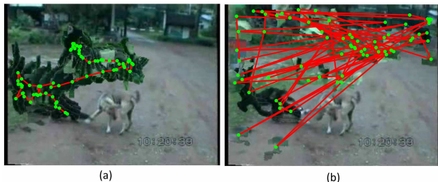
Figure 5. The trajectories of centroids of selected regions, green dots connected with red lines, overlaid over the first frame: (a) when inter-frame mutex constraints are used and (b) when inter-frame mutex constraints are not used.
