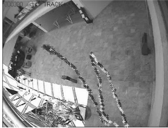
Figure 5 Frame 390 of Walk1 video showing ground truth data and sp motion centroids
