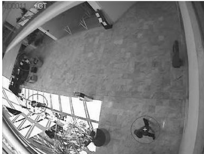
Figure 2 Ground truth data centroids for three objects in frame 11 of Split1 video
