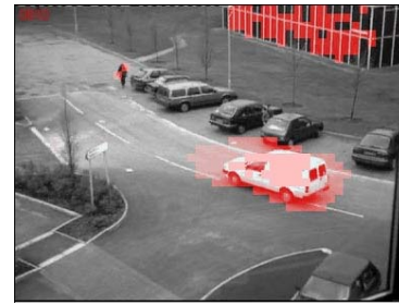
Figure 4. A frame from Campus 3 video with “false motion” artifacts introduced by reflections in the windows.
