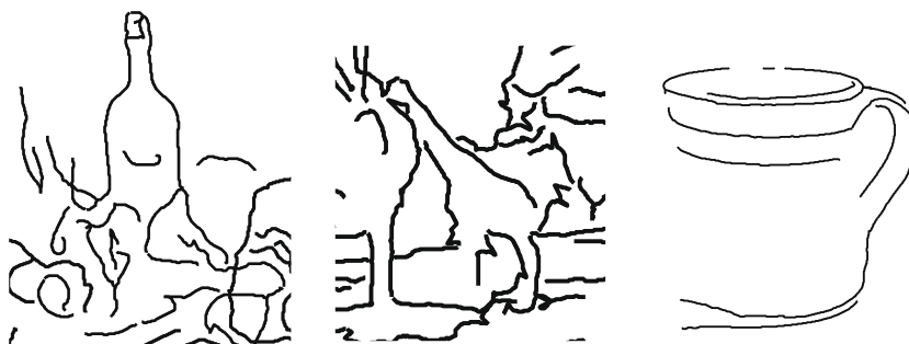
Fig. 4. Parts of the objects are missed both due to missing edge information and due to broken edge links. Objects can still be recognized using shape even if some parts are missing.
