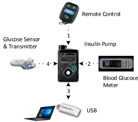
FIGURE 1: A real-time closed-loop control system of insulin pump system.
