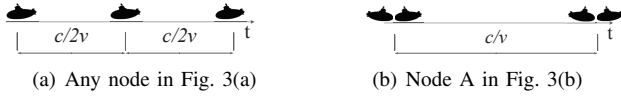
Fig. 4. An illustration of the different movement schedules to the maximal delay. For simplicity, the depth of the sea is 0. The length of the tour is c , and the speed of AUVs is v . In Fig. 3(a), AUV will collect data from sensors every \frac{c}{2v} . However, node A in Fig. 3(b) will be visited by AUVs every \frac{c}{v} .
