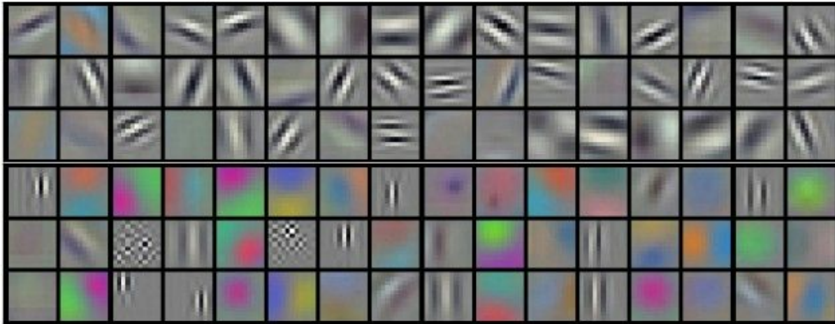
An illustration of the parameters learned in a convolutional layer
