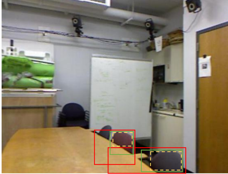
Figure 4.3: Red: two examples of 2D ground truth bounding boxes from [81]. Green: 2D RoI proposals. If compared 2D RoI proposals directly to red bounding boxes, the two positive chair examples are wrongly treated as negative ones. To solve this problem, we added yellow (dashed) gt2d_{sel} boxes for mini-batch sampling.
