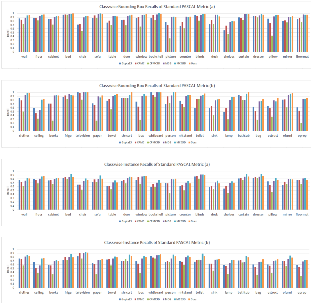
Figure 3.7: Classwise (40-class) performance comparisons based on the standard PASCAL metric (Jaccard Index) at object instance level for both bounding box and segment proposals on the NYU-v2 RGB-D dataset.
