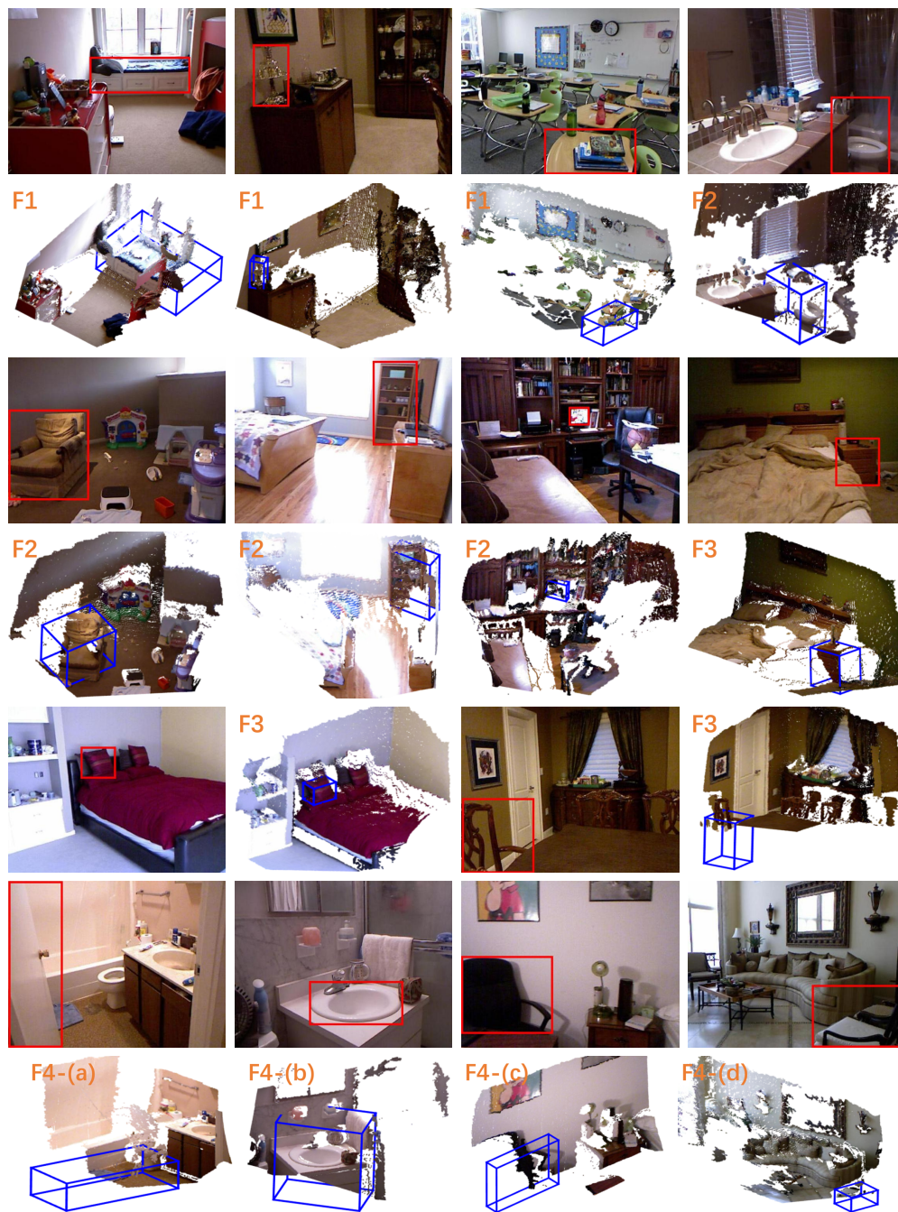
Figure 4.6: Examples of failure cases. 3D detections are rendered in 3D space in blue. The corresponding objects are marked with red bounding boxes. We show four types of failures. F1: box dimension errors. F2: orientation errors. F3: 3D location errors. F4: classification errors ((a) door detected as bathtub, (b) sink detected as toilet, (c) chair detected as tv, (d) chair detected as table).
