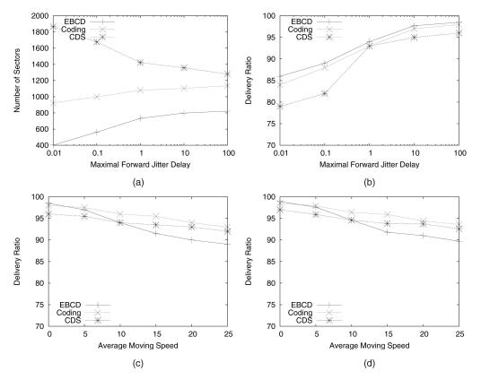
Fig. 14. Performance in a dynamic environment with collision and mobility (K = 4, n = 100). (a) Number of sectors (v = 0). (b) Delivery ratio (v = 0). (c) Delivery ratio in dense network. (d) Delivery ratio in a sparse network.
