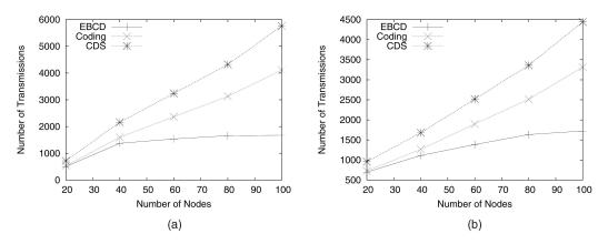
Fig. 10. Comparison of EBCD, Coding, and CDS in number of transmissions. (a) Dense network (d = 18). (b) Sparse network (d = 6).
