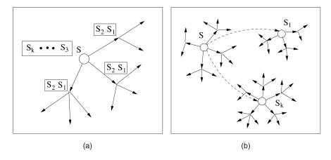
Fig. 9. Single source/single message broadcast. (a) Pipeline-based approach. (b) Spread-out approach.
