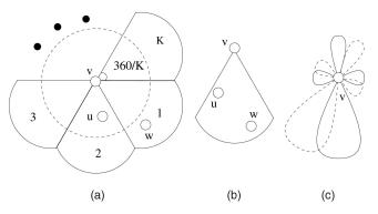
Fig. 2. Directional antenna models in (a) ideally sectorized, (b) adjustable cone, and (c) irregular beam pattern.
